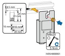
• Method 2: Install the optimizer to the PV module frame using a bolt assembly.
