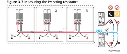
• The measured PV string resistance must meet the following requirement: PV string resistance =  $(R1 + R2)/2 k\Omega \approx N \times 1 k\Omega$ . For example, if there are 16 optimizers in a PV string, the PV string resistance should be about 16 k $\Omega$ .
