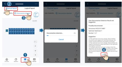
Figure 4-1 Optimizer disconnection detection
