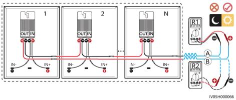
Figure 6-1 Measuring the PV string resistance
